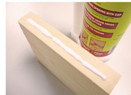
... which is good for edge gluing
