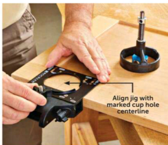
The Rockler jig requires you to measure and mark the location of the cup hole on the door stile, then align the jig with your mark and tighten the clamping knob. The drill guide fits over a raised rim on the base.
