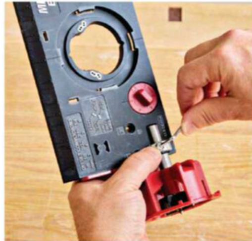
Milescraft provides a depth-stop groove in the base for setting the stop collar. Kreg uses a groove in the bit shank that the set screw aligns with to control boring depth.
